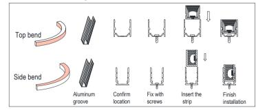
2.Fix with flexible groove
