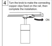
The specific appearance is subject to the real product, Dimming using an integrated adapter (adapter ruler Inch too long).
