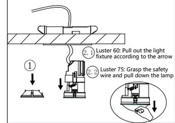
**4.2** Pull out the buckles on both sides to separate the lamp
