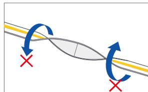
Do not bend LED Strip light like this, and this way will break the LED and bonding pad
