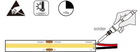
Connecting two welded parts with a maximum temperature of 250 ° C and no more than 5 seconds, and you must wear an electrostatic bracelet.
