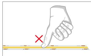
Do not put press heavily or put excessive pressure on surface of LED
