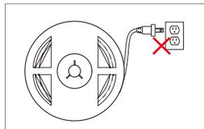
Do not connect directly LED Strip light to AC /DC high voltage power!
