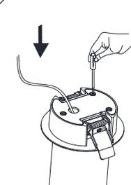
**5** Press the clips on both sides, insert the luminaire into the ceiling.
