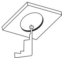
**2** Open the back cover of the luminaire, lead the electricity power supply cable through the back cover.
