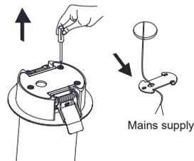
**3** Connect the electricity power supply cable to the terminal block in the luminaire under the condition power off.
