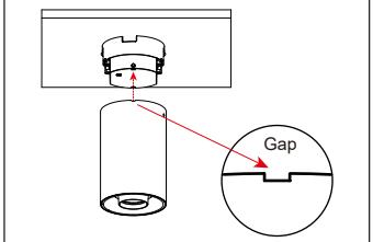
**1.6** Rotate the luminaire clockwise. It installs in place when there is a click sound. Power on to check installation.
