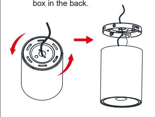
**2.3** Fix the mounting plate by screws.
