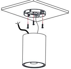
**2.4** Pull out the power supply cable and connect with the light.
