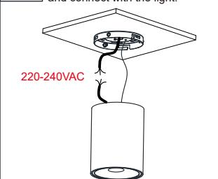
**2.5** Rotate the luminaire clockwise. It installs in place when there is a click sound. Power on to check installation.
