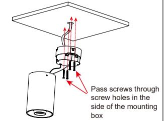
**1.5** Push the luminaire upward with the gap in the top inclined to the prominent chapter in the mounting box
