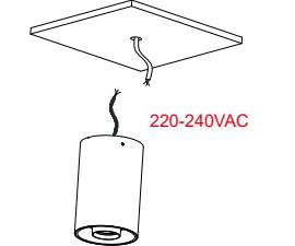
**1.3** Rotate the lamp body counter-clockwise to take out the mounting box in the back.
