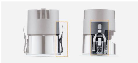
The special springs make the extreme narrow trim possible. The thickness range of ceiling is allowed between 8-20mm.
